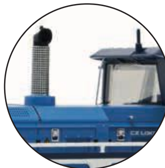
Exhaust pipe panelling made from photo-etched
